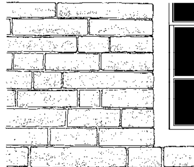
Fig 6. Coursed, squared rubble stonework
